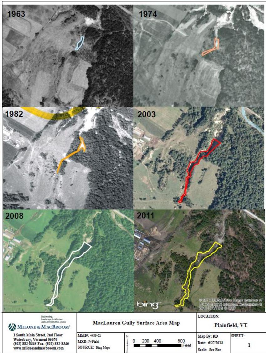
**Figure 12.** This series of maps shows how the MacLauren Gully began in 1963 and has continued to erode and expand significantly in the last 50 years. This project resulted in the first of its kind in Vermont landslide hazard map.
